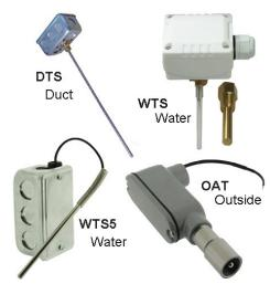
There are several sensor element ranges to choose from, which guarantee compatibility with all popular DDC systems. The sensor elements are precision thermistors or platinum RTDs. Field calibration is not generally required. The probe is epoxy sealed to prevent moisture from migrating into the probe. Custom probe lengths, wire types and sensor elements are available for large OEM projects. Ask about our plastics & metal manufacturing capabilities for custom housings as well.
