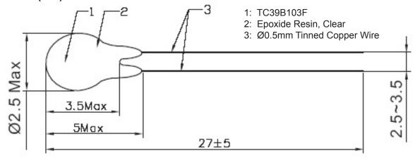
RTS-Bead-4: Thermistor bead, 4"(10cm) lead, 10mm wire trimmed and tinned, 0.2DegC accuracy
