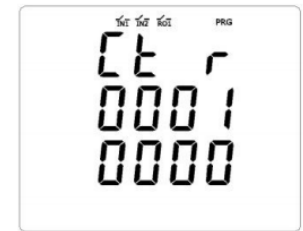
Current Transformer Ratio
