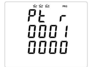
Potential Transformer Ratio
