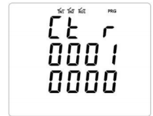
Current Transformer Ratio
